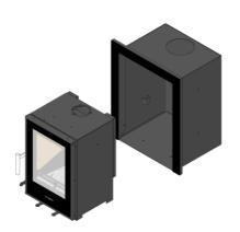
4. Remove inner stove from outer shell – Remove all vermiculite bricks from stove and remove internal bolts either side of stove chamber.
